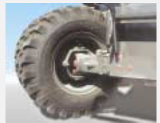
The oil-bath multi-disc brakes ensure gentle yet effective braking response. The brakes themselves need no adjustment.
