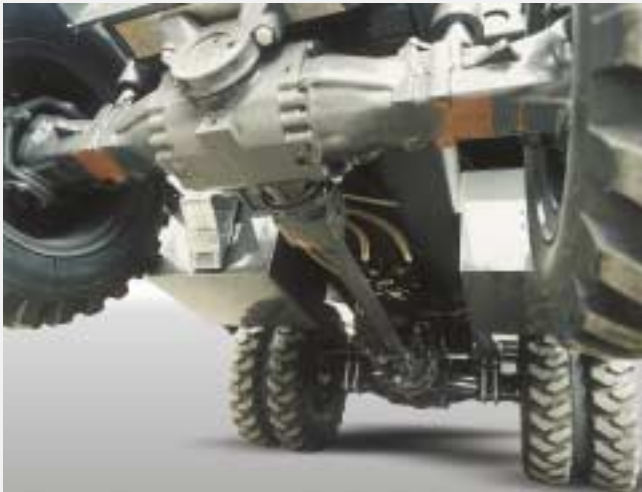
Generous ground clearance for excellent terrainability. The front axle oscillates (14°) and is hydraulically lockable at any angle.
