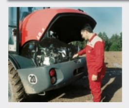
The large engine hood opens up widely and easily, and all the components are readily accessible. Routine daily maintenance is completed in no time at all. The slim patented longitudinal beam permits easy accessibility, from the
