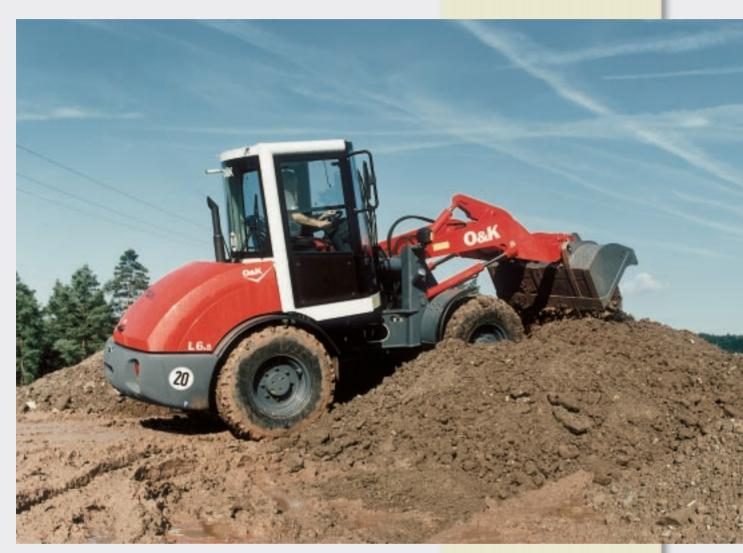
$\begin{tabular}{lll} L 6.5 & L 8.5 \\ \hline Service weight & 4.7 t & 5.1 t \\ \hline Engine output & 42 kW & 44 kW \\ Loading buckets & 0.8 m³ & 0.9 m³ \\ \hline \end{tabular}$
