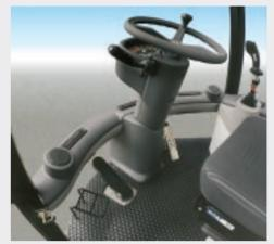
ed fresh-air blower ensures an agreeable working climate. The multipurpose lever conveniently controls lifting, lowering, rollback, dump and reversing-under-load functions. Single-handedly! All this speeds up work.
