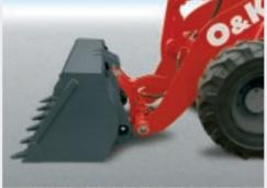
The elastic bucket stop absorbs noise for reduced stress on material, operator and environment.
